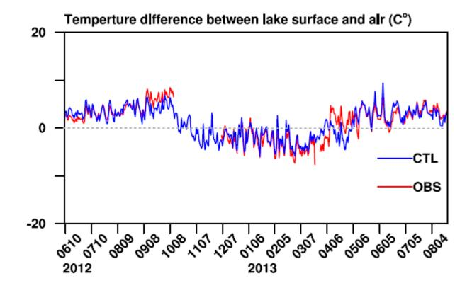
The model could represent the temperature difference between lake surface and atmosphere in ice-free period.
