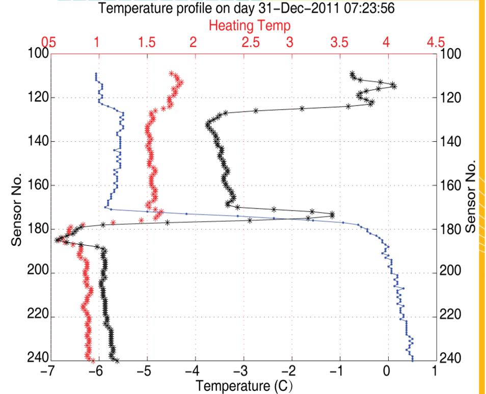
Left: Temperature profiles of one SIMBA measured in Svalbard. The black lines are interpolated /extrapolated linear temperature gradients.
