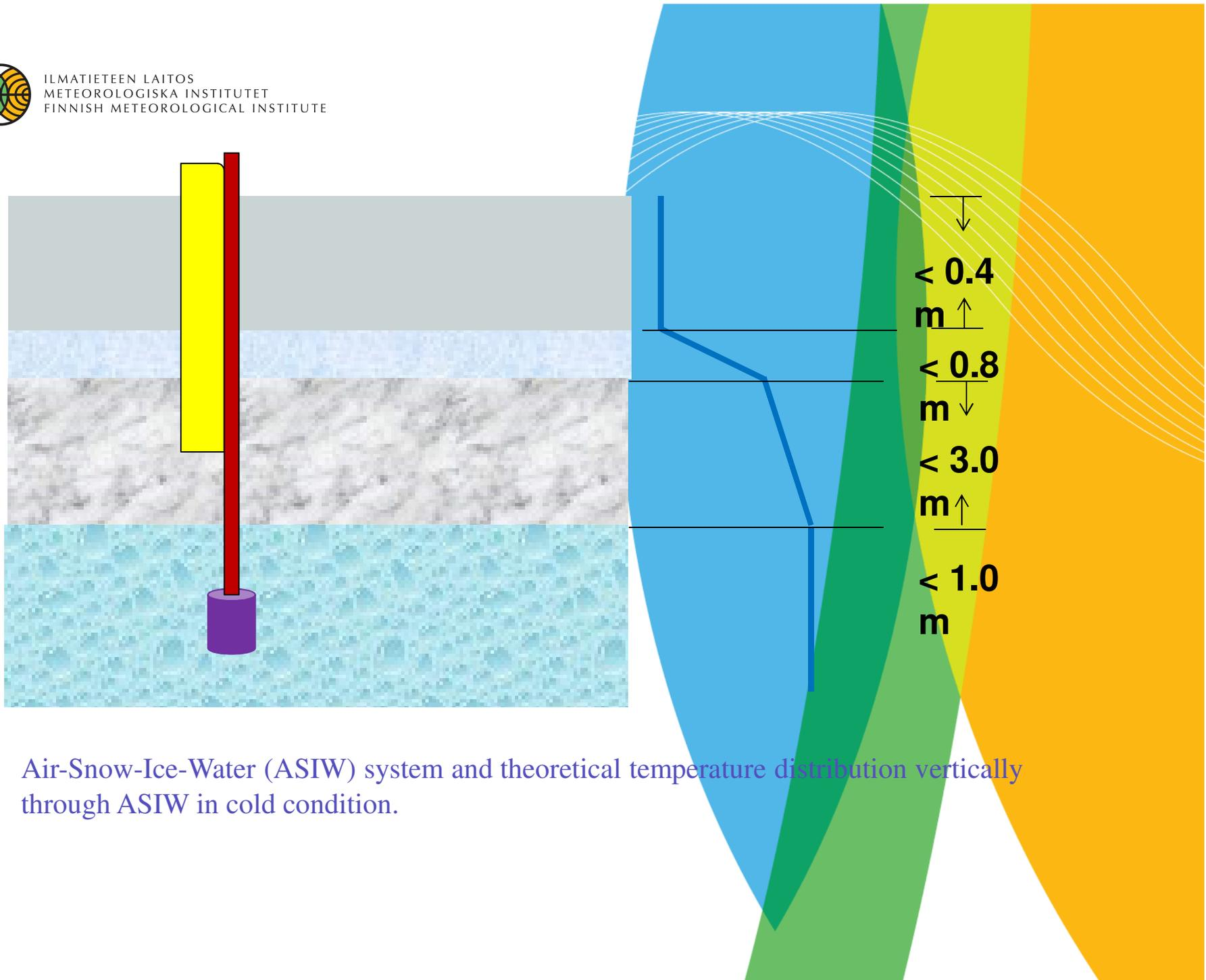
Air-Snow-Ice-Water (ASIW) system and theoretical temperature distribution vertically through ASIW in cold condition.
